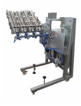
The destacker with suction cups (DMF) has been designed to put products or box containers on conveyor belt.
